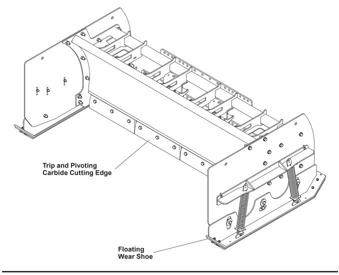
Your pusher plow ships from the factory with the trip and cutting edges already installed and the wear shoes pre-assembled to the side plates. To complete the snowplow assembly follow the steps below.
