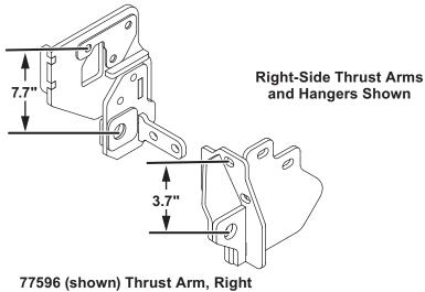
77596 (shown) Thrust Arm, Right 77595 (not shown) Thrust Arm, Left 77598 (shown) Hanger, Right 77597 (not shown) Hanger, Left
