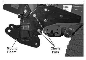
NOTE: After five to ten hours of snowplow usage, retorque all mount assembly fasteners.
