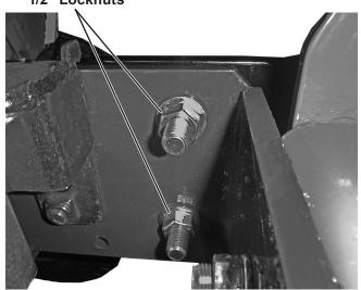
3. Install one 3/8" x 2-1/2" cap screw through the middle hole of the left hand side plate and frame rail as shown. Secure with a 3/8" washer and 3/8" locknut and hand tighten.
