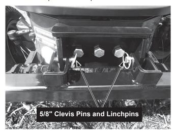
5. Secure the rear arms of the mount beam to the lower lugs of the tractor using two 5/8" clevis pins. Secure each clevis pin with a linchpin. It may be necessary to loosen the front mount plate fasteners and reposition the front mount plate to allow the holes in the rear arms to align with the lower lugs of the tractor. Then tighten the front mount plate fasteners again.
