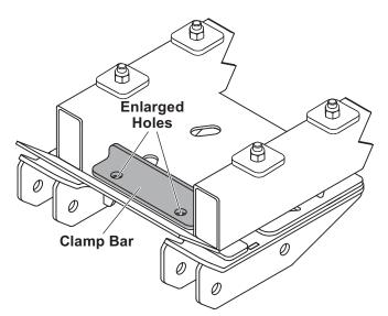
Place a 3/8" washer on each of two 3/8" x 1-1/4" cap screws. Install the fasteners up through the center holes of the skid plate assembly, vehicle frame, and clamp bar. Secure the fasteners with 3/8" locknuts. Hand tighten.
