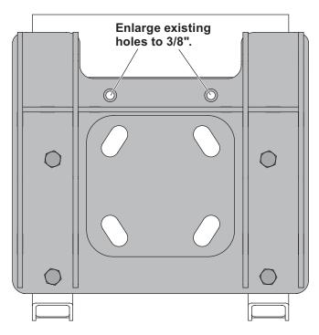
5. Install the clamp bar on the inside surface of the vehicle's frame, positioned over the holes enlarged in Step 4.
