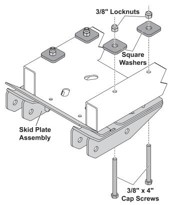
4. Using the center holes of the skid plate assembly as a guide, enlarge the existing holes in the vehicle frame to allow 3/8" fasteners to pass through.
