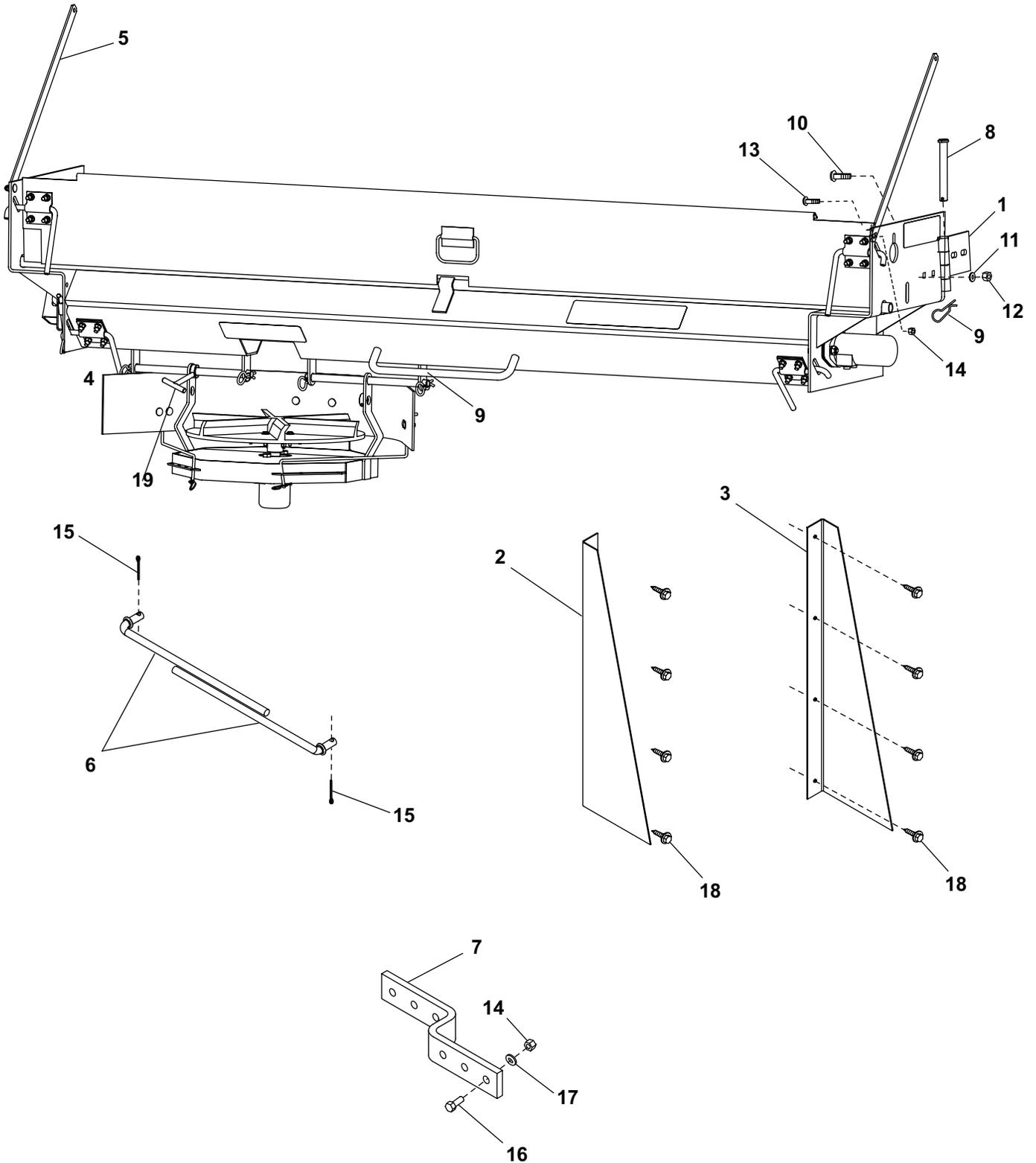
This parts list is for UTS 696 Under Tailgate Spreaders with serial numbers 0216 and higher.
