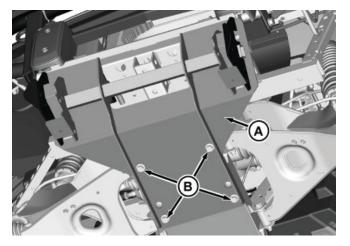
Loosely install four M12 x 30 flanged cap screws (B) through the blade frame and into the nut bars.  Loosely attach the upper part of the blade mount (A) to the vehicle frame (B) with an M12 x 30 flanged cap screw (C) and M12 flanged locknut (D).
