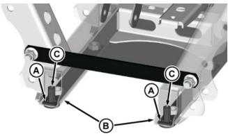
2. Install bracket (A) through the holes in the bottom of the frame (B).
