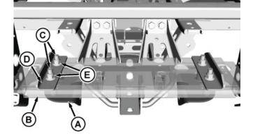
3. Insert two M12 x 80 flanged cap screws (C) from the bottom through the bracket (A).
