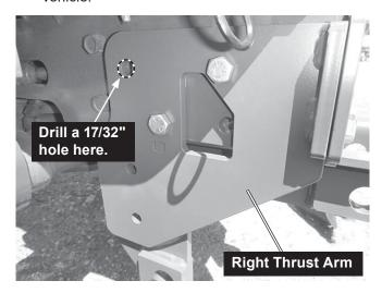
10. Tighten all fasteners according to the torque chart.
