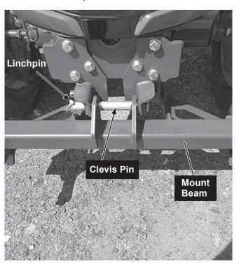
15. Install the 1" x 2-3/4" clevis pins through the mount beam and thrust arms. Secure with the provided linchpins. Install the removable mount beam using the 1" x 8" clevis pin through the front mount assembly and push beam, and secure with a provided linchpin.
