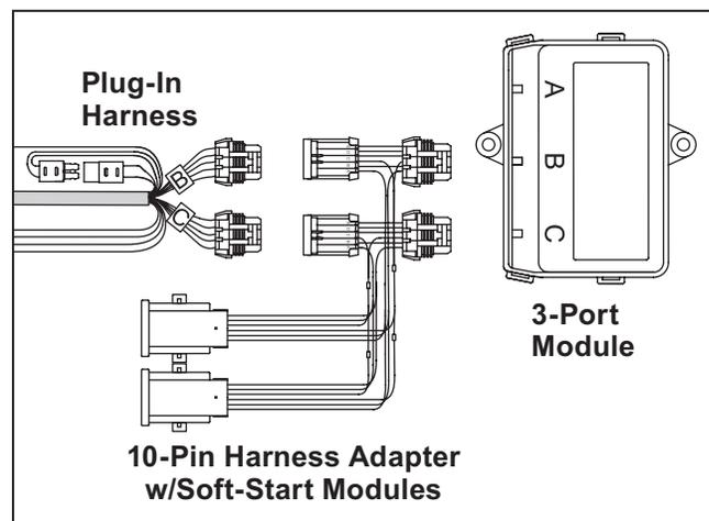
2. Mount the soft-start modules in an area that receives good airflow, such as the cavity between the grille and the radiator.
