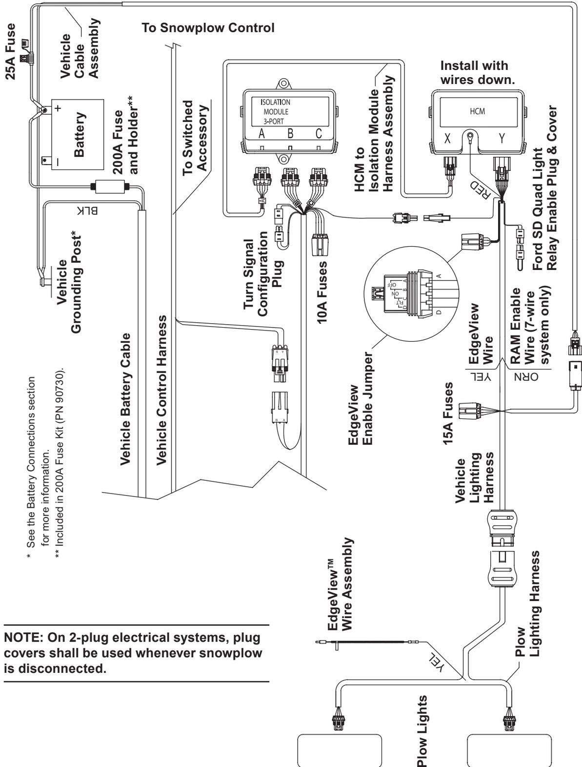
**NOTE: On 2-plug electrical systems, plug covers shall be used whenever snowplow is disconnected.**
