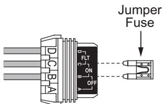
**FLT:** Blade edge lights illuminate when blade is in FLOAT mode.
