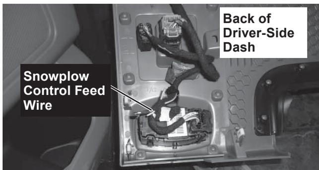
8. Route the red "ACC" wire from the vehicle control harness to this location and trim away excess length.
