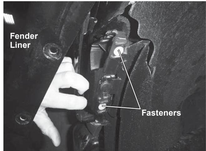
2. To remove the headlamp assembly trim panel, start by removing the fasteners shown.
