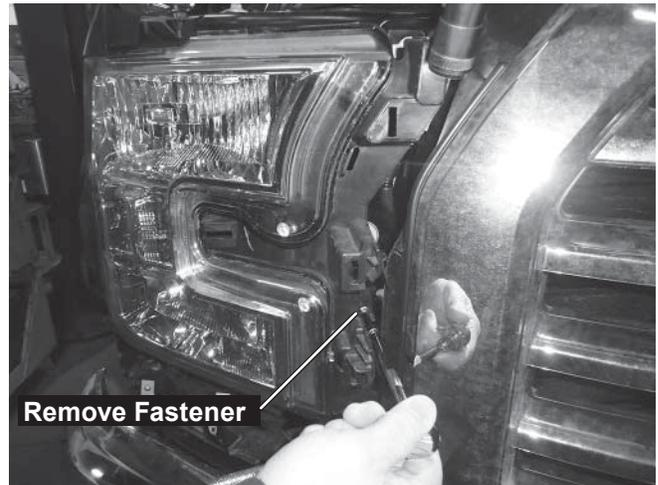
10. Remove the two fasteners on the top of the headlamp assembly.
