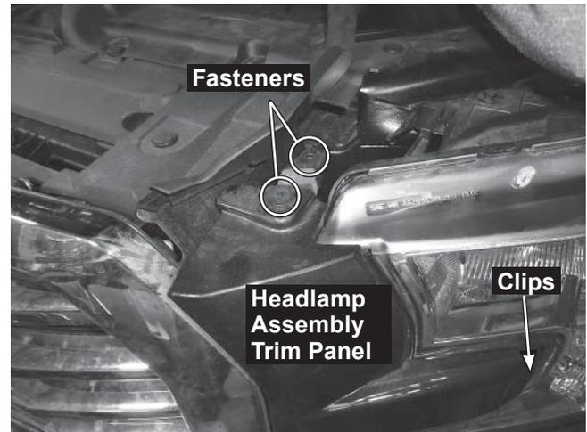
3. From the inner edge, release the headlamp assembly trim panel clips. Start at the outer edge of the assembly to release the headlamp assembly trim panel.
