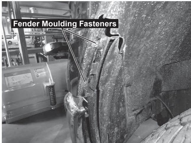
2. Release the three fender moulding locks and partially remove the fender moulding.
