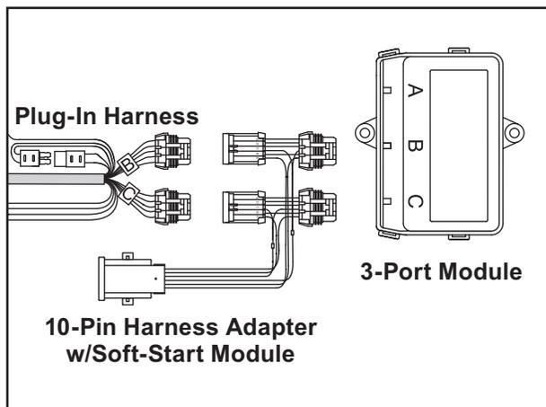
**For vehicles with headlamp bulb or turn signal daytime running lights (DRLs):** The DRL wire from the plug-in harness will not be used. Coil and cable tie the DRL wire.
