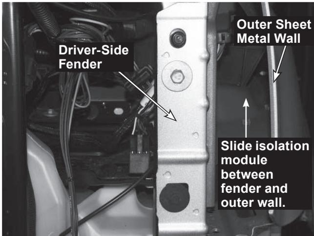
Install the isolation module on the inside of the driver-side fender using the supplied cable ties, reclosable fastener strips, and edging material as shown below.
