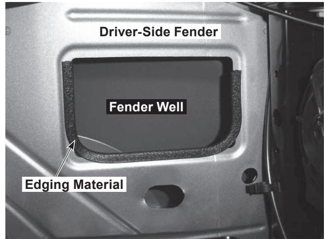
4. Remove the cable clip currently in place above the fender well. Drill a 5/16" hole approximately 1/2" above the existing cable clip hole.
