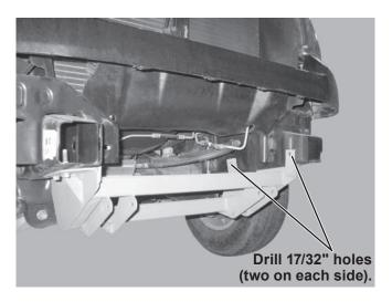
8. Place a 1/2" washer onto a 1/2" x 1-1/4" cap screw with handle, and insert the cap screw into the truck frame. Pass the cap screw out through the hole in the truck frame and the hole in the rear tab of the mount. Place a 1/2" locknut on the cap screw and hand tighten.
