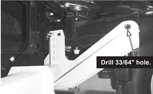
8. Using the remaining slotted holes as guides, drill  $33/64$ " holes through the frame.
