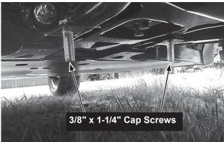
5. Place the skid plate assembly against the vehicle frame, allowing the fasteners installed in Steps 3 and 4 to pass through the assembly. Secure all four cap screws with 3/8" locknuts; hand tighten.
