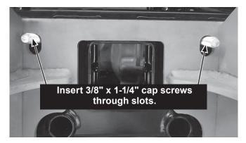
Secure cap screws with 3/8" washers and 3/8" locknuts. Hand tighten.
