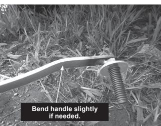
4. Install two 3/8" x 1-1/4" cap screws down through the holes of the rear A-arm bracket, located just forward of the rear A-arm.
