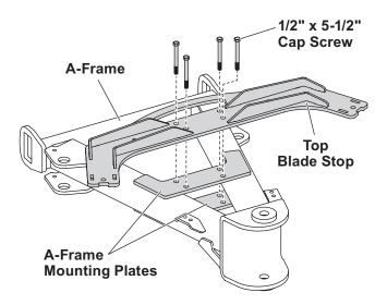
2. Insert four 1/2" x 5-1/2" cap screws through the holes in the top blade stop and the A-frame mounting plates.
