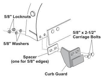
**Carbide Edges:** For all carbide edges, install two spacers between the curb guard and blade.
