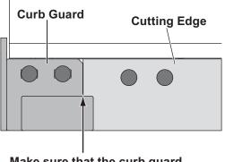
Make sure that the curb guard is flush against the cutting edge.
