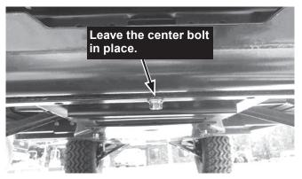
3. Insert two 3/8" x 5" cap screws into each rear bracket. Place the brackets over the frame, one on each side of the vehicle in the location shown.
