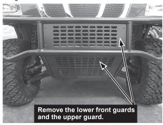
2. Remove the left and right lower brush guard assembly bolts found underneath the vehicle. Leave the center bolt in place.
