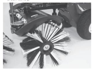
6. In the center, the tab on the cap-gear should fit the slot on the brush cylinder.
