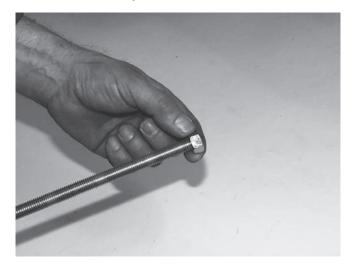
2. Put cap, washer, and locknut on the axle.
