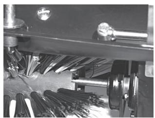
8. Put the cap and washer on the end. Thread on locknut.
