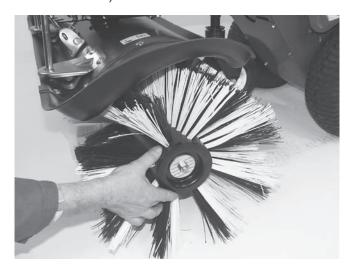
5. Put the axle with the cap, washer and brush through the drive source (centered underneath the brush cover).
