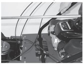
2. Mount handlebar to the supports with the knob.
