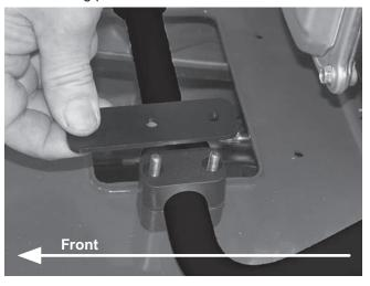
5. Put M6 locknut and washer on the stud.
