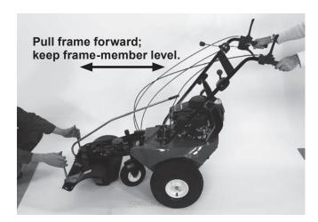
3. Loosely preassemble the brushing subassembly to the axle drive housing with cap screws and washers. Begin at the front.
