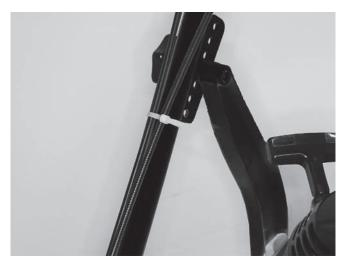
The ties here must form a loop. Do not tighten completely. The cable must be able to move when the handle is folded.
