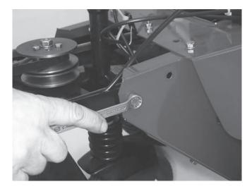
Remove the cap screws on both sides that hold the wheel drive housing to the brush drive frame. Pull the brush drive frame forward keeping the frame-member as level as possible and keeping the frame from scraping the cover. DO NOT REUSE THE REMOVED HARDWARE.
