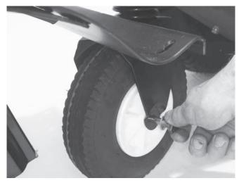
5. Use two 17 mm wrenches to tighten the fasteners.
