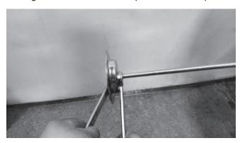
4. Put the axle with the cap, washer and right brush through the drive source (centered underneath the brush cover).
