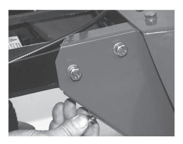
4. Use a 13 mm wrench to tighten the fasteners that hold the brushing mechanism to the axle drive housing. Tighten in the order shown.
