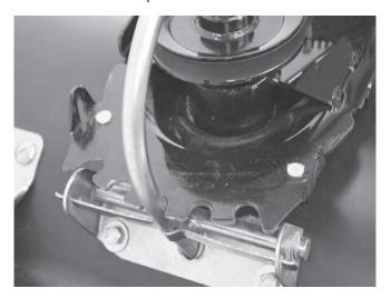
13. Set the brush at an angle. Slip the cover over the belt area and back so the snap Nuts can be seen through the holes in the cover.
