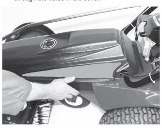
14. Put TORX® screws with the countersink washers through the mounting holes on the cover and thread into the snap nuts.
