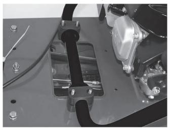
4. Put fixing plates on the studs. Position as shown.
