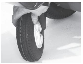
4. Push the M10 x 100 mm cap screw through and thread on the nut. Use a 17 mm wrench.
