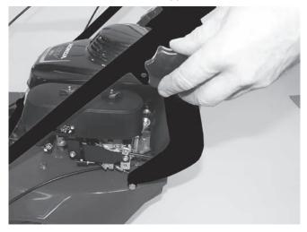
3. Put the other half of the clamps onto the studs.
