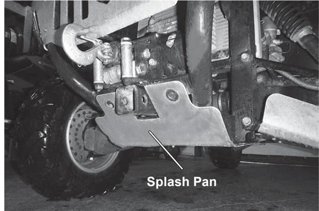
2. Remove and retain the two lower fasteners.
