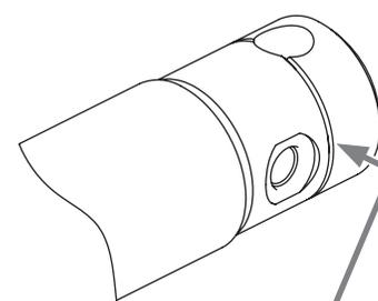
Current rams have a groove all around the base, near the pin hole. Early rams do not have a groove.
