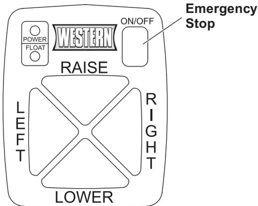
1. Turn the vehicle ignition switch to the ON or the ACCESSORY position. The control logo area will become illuminated.
