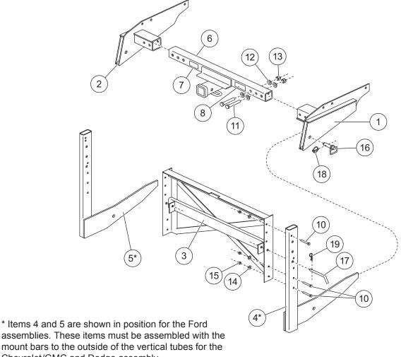
assemblies. These items must be assembled with the mount bars to the outside of the vertical tubes for the Chevrolet/GMC and Dodge assembly.
