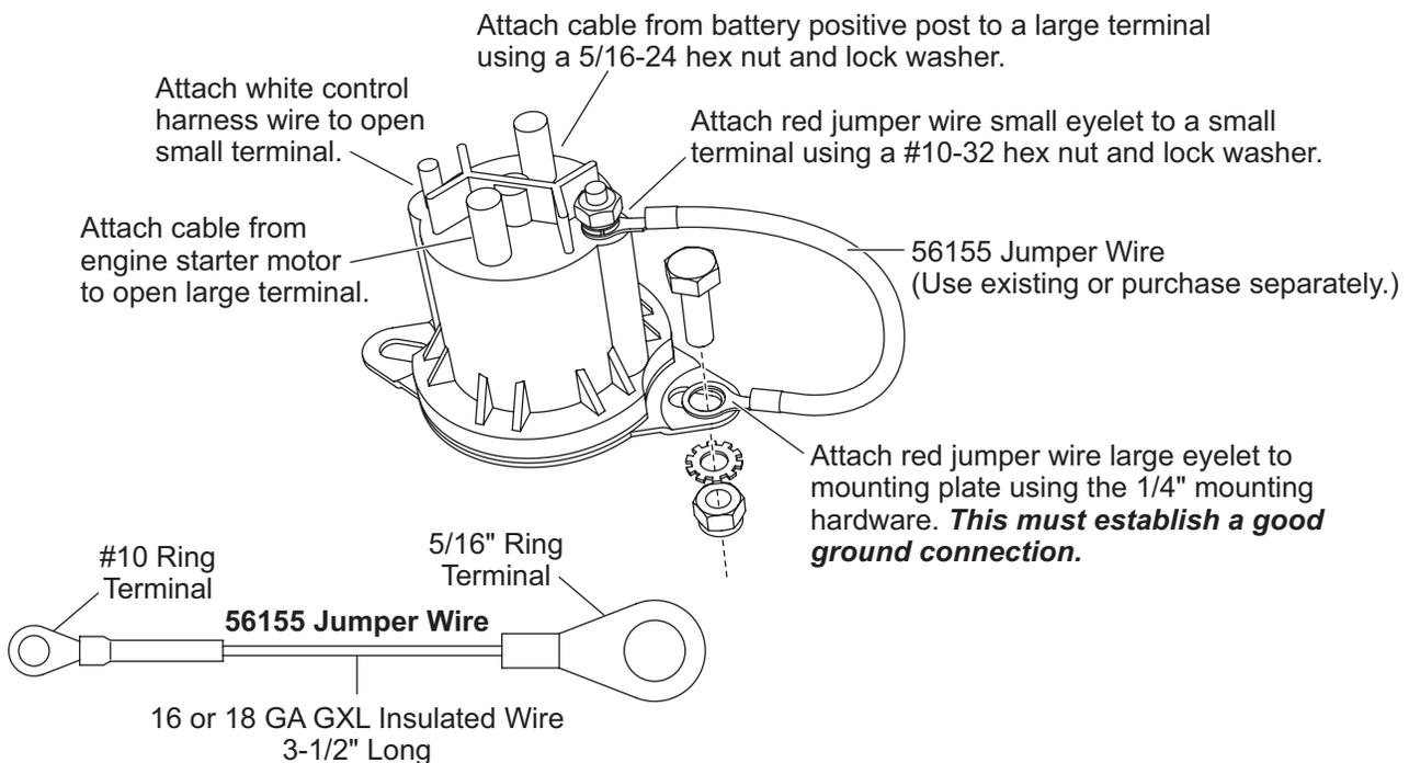
**NOTE:** Overtightening terminal attaching nuts may cause seal failure, resulting in premature failure of this relay.
