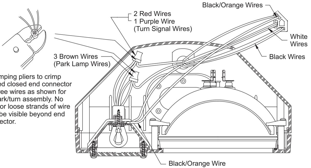
Use crimping pliers to crimp furnished closed end connector onto three wires as shown for each park/turn assembly. No copper or loose strands of wire should be visible beyond end of connector.
