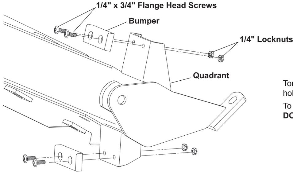
Torque Locknut to 35 in/lb while holding screw.
