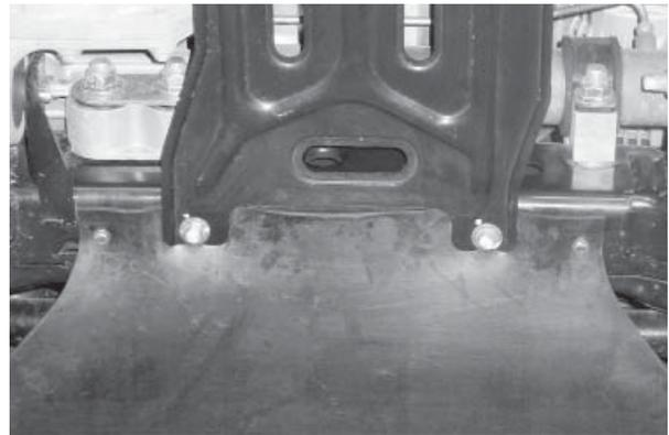
**If the vehicle is not equipped with a transaxle skid plate**, align the holes in the rear splash shield retainer and the tapered end of the splash shield with those in the vehicle frame cross member. Install two M6 x 1.00 cap screws and flat washers (supplied with the mount) through the rear splash shield retainer and splash shield and into the cross member. Do not overtighten.
