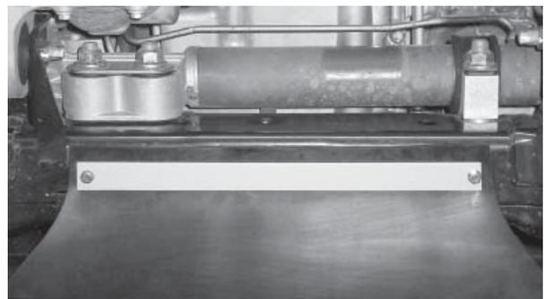
5. Make sure the splash shield is under the vehicle sway bar, then pull the uncut end of the shield to the vehicle bumper support beam.
