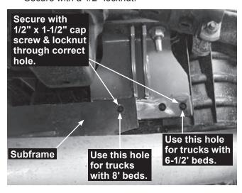
4. Install 1/2" x 1-1/2" cap screws in remaining locations and secure with 1/2" locknuts.
