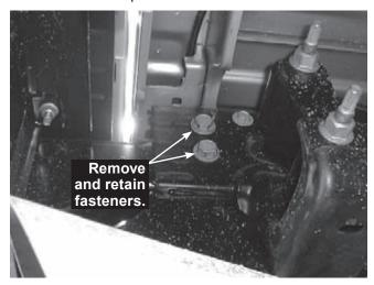
Install the rear bracket as shown. Secure the bracket with the original bumper fasteners. Finger tighten.
