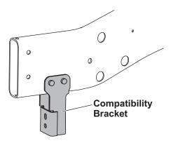
3. Remove the nuts from the bumper fastener assembly on both sides of the vehicle. For both driver-side and passenger-side mounts, align the forward mount holes with the protruding cap screws and guide the mounts onto the respective bolt assembly. Loosely fasten by reinstalling the original nuts.
