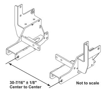
Tighten the M10 stabilizer bracket cap screws and all remaining fasteners according to the torque chart. Start at the front of the mount and work rearward.
