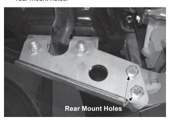
Thrust arms are interchangeable and can install on either side of the vehicle. There is no left or right side-specific part.
