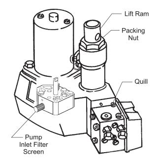
Periodically verify the lift ram and the Hydra-Turn™ ram packing nuts are tight.
