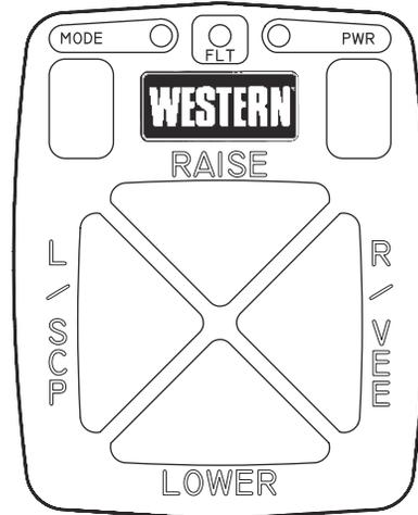
2. Press the PWR button on the control. The control indicator light will glow red indicating the control is on. The control indicator light will glow red whenever the control ON/OFF switch and the vehicle ignition switch are both ON and the plow plugs are connected to the grill connectors.
