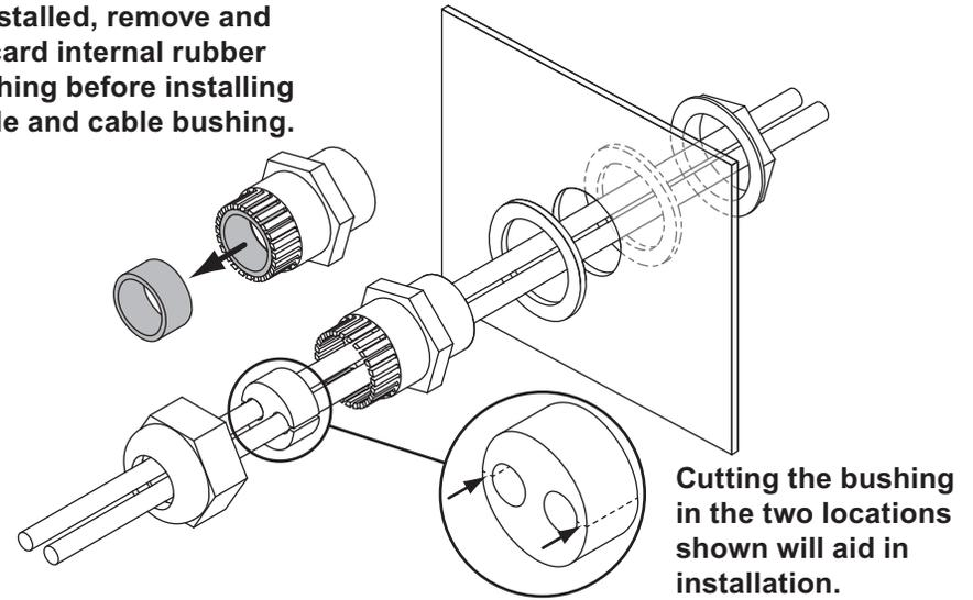
Cutting the bushing in the two locations shown will aid in installation.
