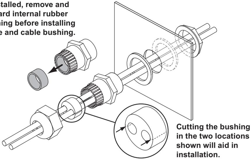
Cutting the bushing in the two locations shown will aid in installation.
