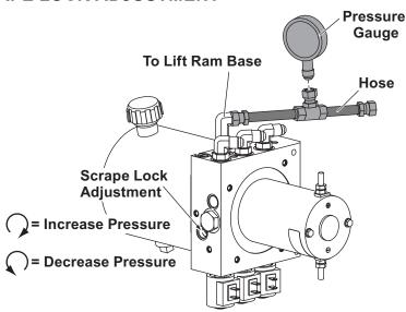
Follow the instructions below to increase the pressure setting of the scrape lock feature. The snowplow must be attached to the vehicle, and the snowplow battery cable and lighting harness must be connected before beginning this procedure.
