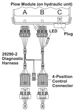
Connect the diagnostic harness connectors A and B to the matching ports on the plow module (A to A and B to B).
