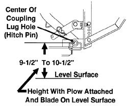
4. Adjust chain slack with plow mounted to vehicle and lift channel pushed all the way down. To adjust, remove chain from hook. Straighten chain and pull tight. Rehook it to lift channel. After it is hooked, it will have the correct amount of slack for blade "float." DO NOT remove chain from lift channel when removing plow from vehicle.
