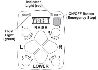
Press the ON/OFF button on the control. The power indicator light glows red, indicating the control is ON. The indicator light glows red whenever the control and the vehicle ignition switch are both ON and the electrical connections to the snowplow are completed.
