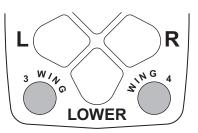
The two round buttons located to the left and right of the LOWER button move either wing independently of the other as described below.
