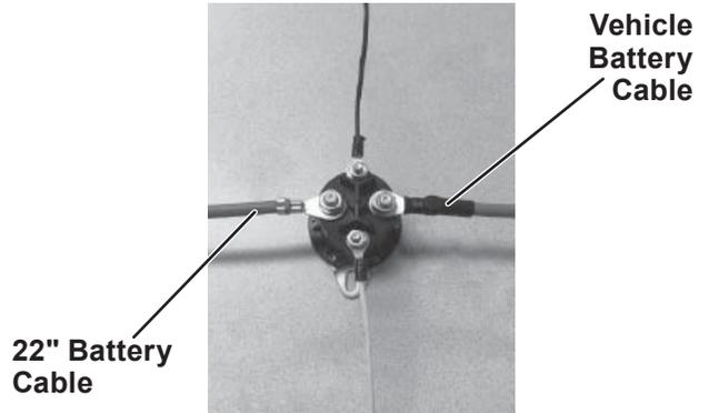
11. Connect the spreader cable (PN 66425) to the vehicle cable (PN 66242).
