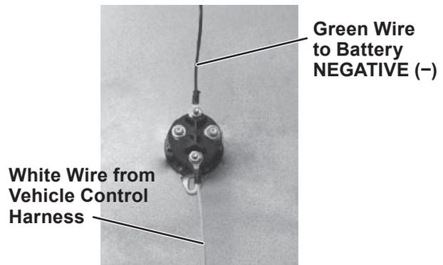
3. Verify that the wire is protected or secured away from all sharp edges and hot or moving parts
