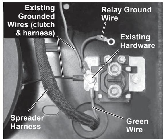
2. Connect the white wire from the spreader harness to one of the primary (small) terminals of the starter relay and connect the relay ground wire to the other small primary terminal on the relay.
