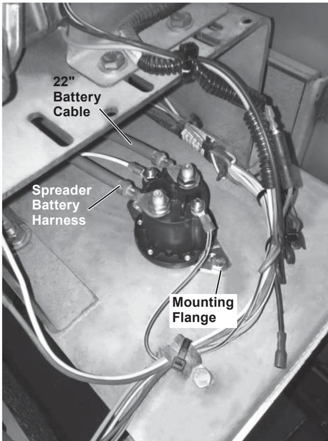
2. Install the red battery cable (PN 66246) to one of the large secondary terminals of the starter relay and to the POSITIVE (+) battery terminal.
