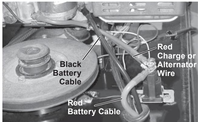
6. Connect the red battery cable (PN 65246) to the POSITIVE (+) terminal of the battery.
