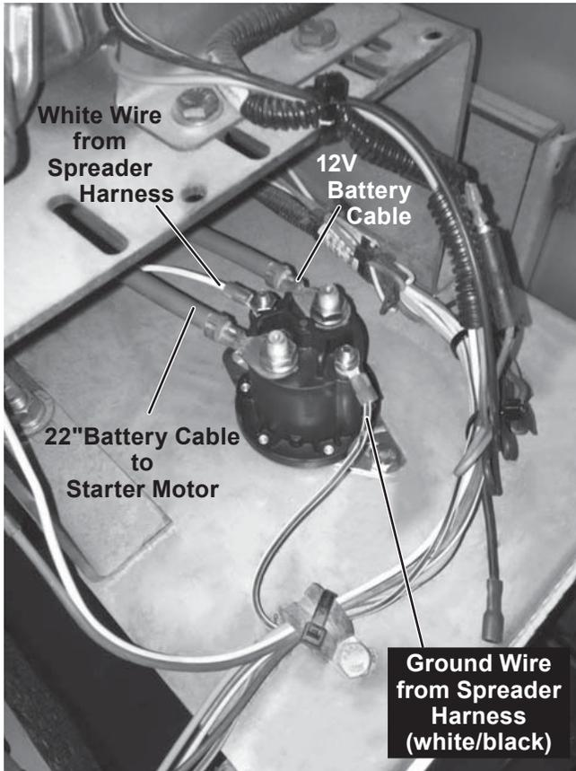
7. Verify the black wire from the spreader harness to the engine shut-off circuit is connected.
