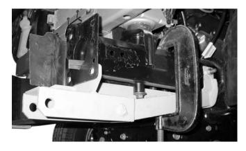
11. Realign the bumper assembly with the vehicle for proper appearance. Tighten the two uppermost outer fasteners to hold the bumper in alignment. Measure the distance between the vehicle mount U-brackets. Adjust this distance to be 30-7/16" ± 1/8" center-to-center, and tighten the six remaining bumper fasteners according to the torque chart.
