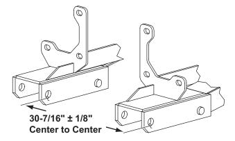
12. Tighten the four fasteners to the rear of the mount according to the torque chart.
