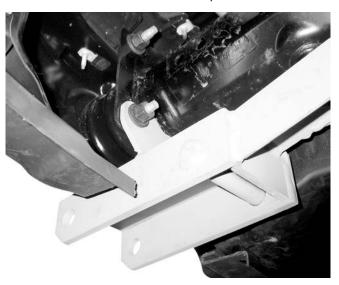
4. Hold the mount tight to the bottom of the frame using a clamp or a floor jack.
