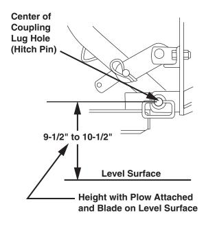
NOTE: Coupling height must be 9-1/2" minimum to allow stand to be pinned to frame.
