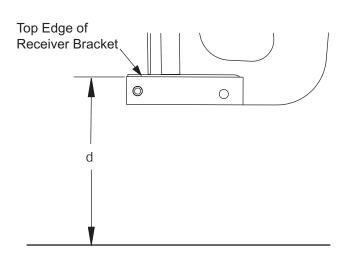
Prior to assembling the kit, measure the distance from the top of the UniMount receiver bracket to the ground. Assemble the items shown on the parts list in the position shown in the following diagrams.
