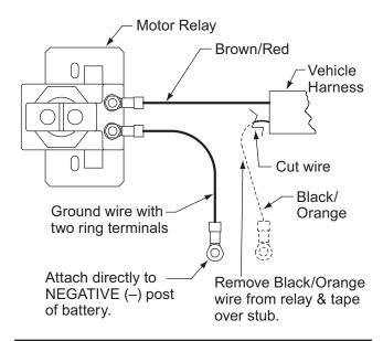
NOTE: Before plugging in the control, proceed to the Control Ground Modification Instructions. Failure to do so will result in grounded headlamp relays, which will cause the vehicle headlamps to remain OFF when the snowplow is removed.
