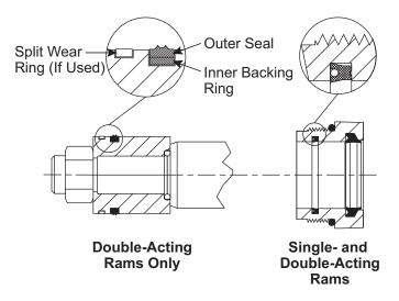
3. **For single-acting rams:** Slide gland nut over split bearing end of rod to prevent damaging seals.
