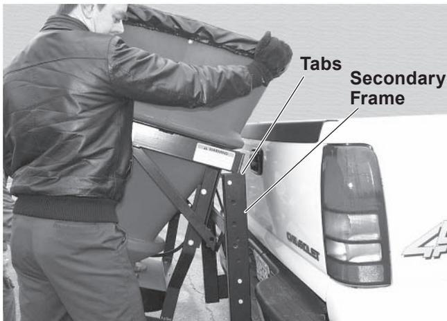
2. Allow the spreader assembly to rotate until the bottom contacts the secondary frame assembly.
