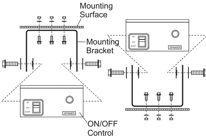
1. Locate a convenient position in the cab to mount the control that will not interfere with other equipment and will avoid unintentional starting of the spreader.
