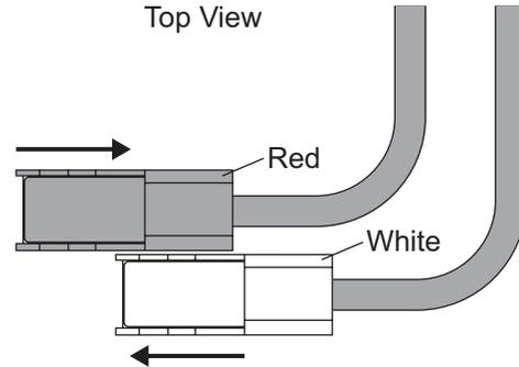
5. Plug the 2-way molded connector from the vehicle wiring harness into the matching connector extending from the rear of the cab control as shown below.
