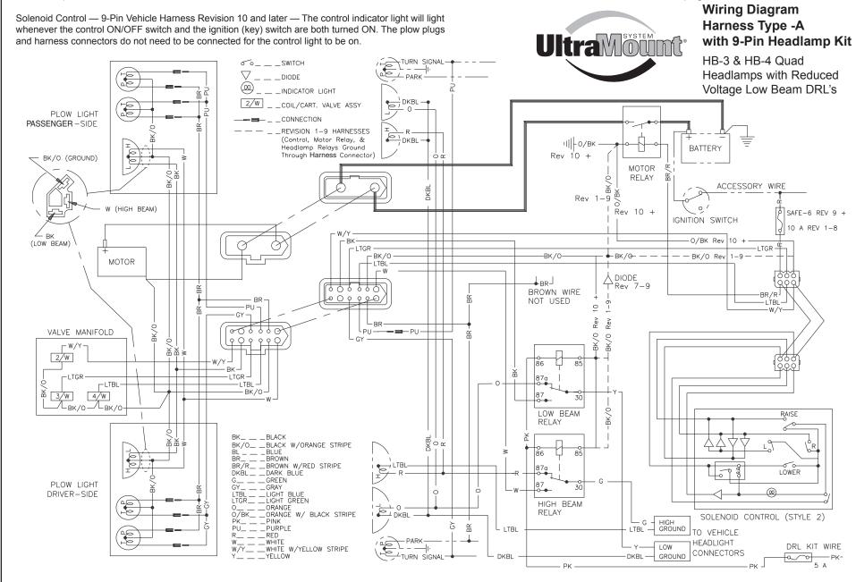
9-Pin Vehicle harnesses — P.N. 61437, rev. 7, 8, or 9 — The indicator light on the solenoid control will only light when both plow plugs and harness connectors are connected and the ignition (key) switch and control on/off switch are both turned on.
