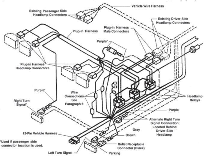
**REMINDER:** Lubricate all receptacles and blades with dielectric grease before assembling.
