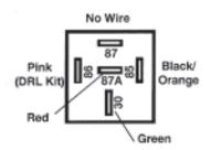
Vehicle High Beam Headlamp Relay
