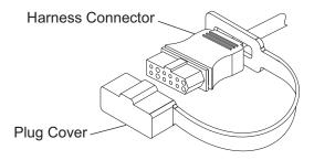
6. Find a location in the vehicle bumper/grill area on the battery side for mounting the battery cable harness connector. The best location is at least 10-1/2" from the center of the grill and at a convenient height for connecting the plow plugs.
