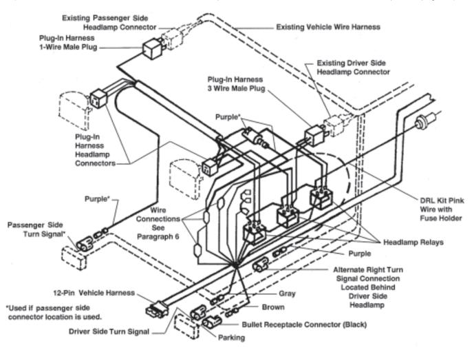
**REMINDER:** Lubricate all receptacles and blades with dielectric grease before assembling.
