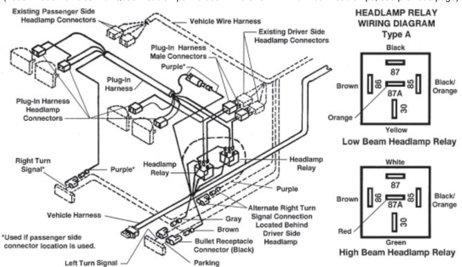
**REMINDER:** Lubricate all receptacles and blades with dielectric grease before assembling.
