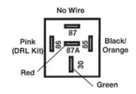
Vehicle High Beam Headlamp Relay
