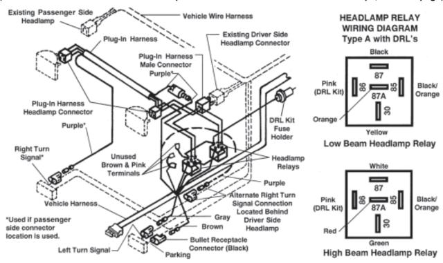
**REMINDER:** Lubricate all receptacles and blades with dielectric grease before assembling.
