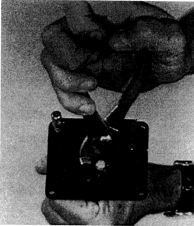
Step 41: Using pliers, lightly compress the tangs on the cable conduit snap fitting.
